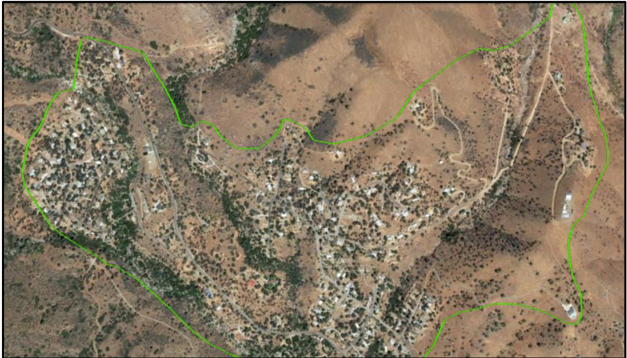
Figure D.46. Community is intersected by highway 155 and Earl Pascoe Road. Limited fire access with extremely steep slopes and limited turnarounds. Many homes perched mid slope.
